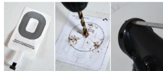
Mounting is easy, thanks to the supplied template. Non-wireless phones can use a separate receiver
